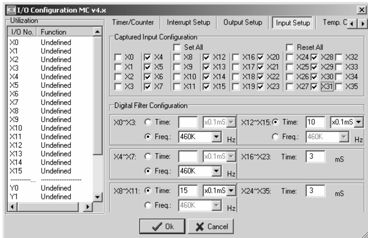
The FBs series PLC can support up to 36 points of captured input (X0~X35) depending on the main unit. The inputs X0~X15 can be configured as the hardware interrupt input for fast response application, and the captured inputs are for low frequency but short duration (less than 1 scan time) input signal.
