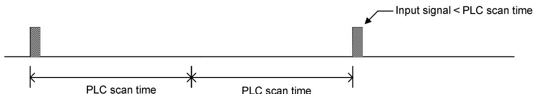
The FBs series PLC main unit supports the captured input function as mentioned above, except this, it also supplies the digital filtering function for digital inputs X0~X35. There are 6 groups of digital inputs { (X0~X3)、(X4~X7)、(X8~X11)、(X12~X15)、(X16~X23)、(X24~X35) } for filtering setting.
