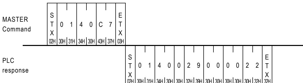
● Command code 41 (Control the PLC RUN/STOP)
