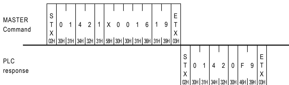
● Command code 43 ( The status reading of ENABLE/DISABLE of continuous discrete )
