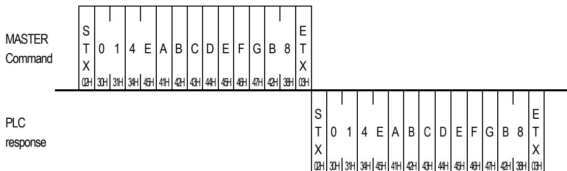
● Command code 53 ( Read the detailed system status of PLC )
