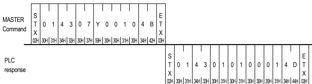
● Command code 44 (The status reading of continuous discrete)
