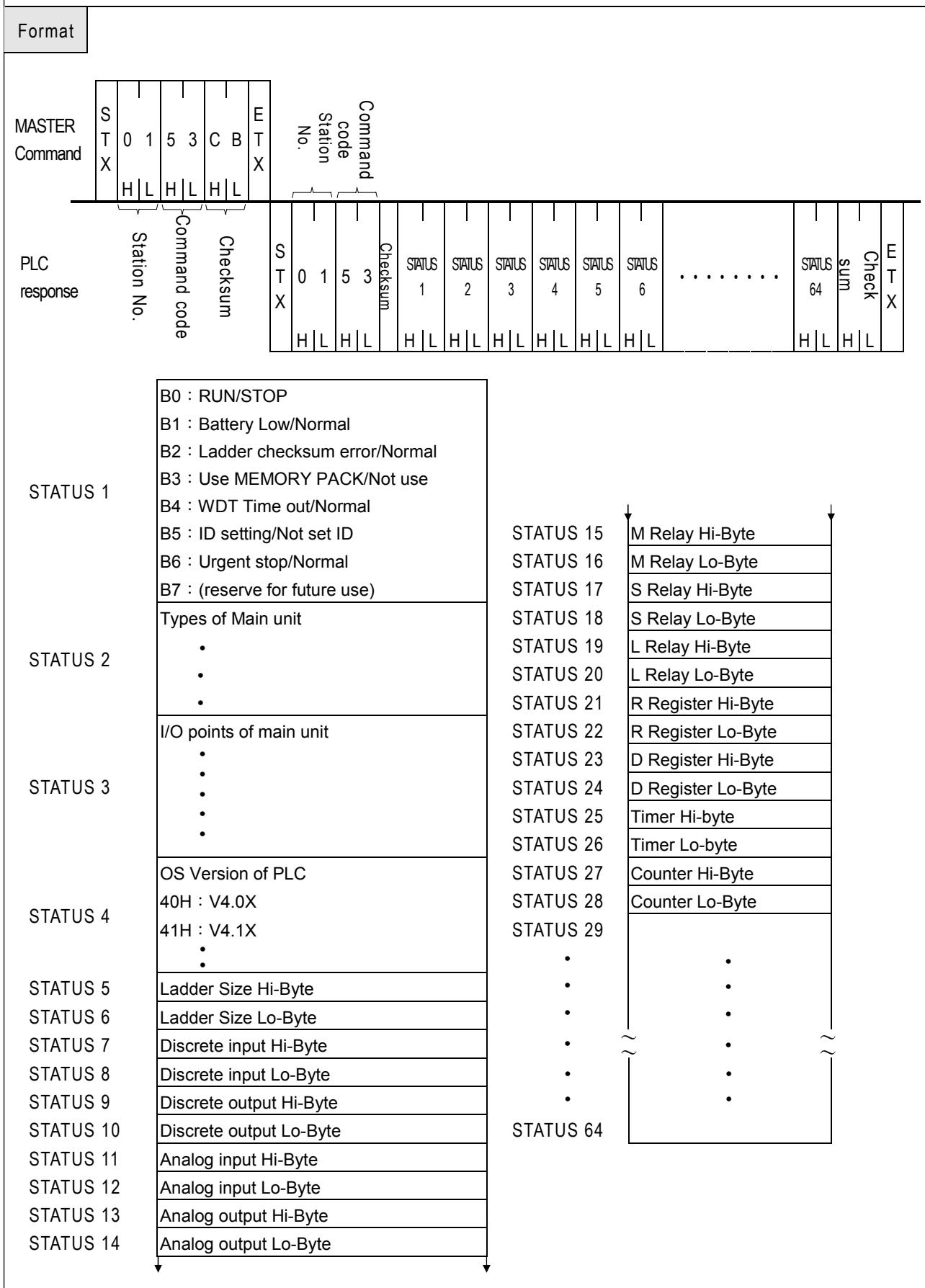
● Command code 53 ( Read the detailed system status of PLC )
