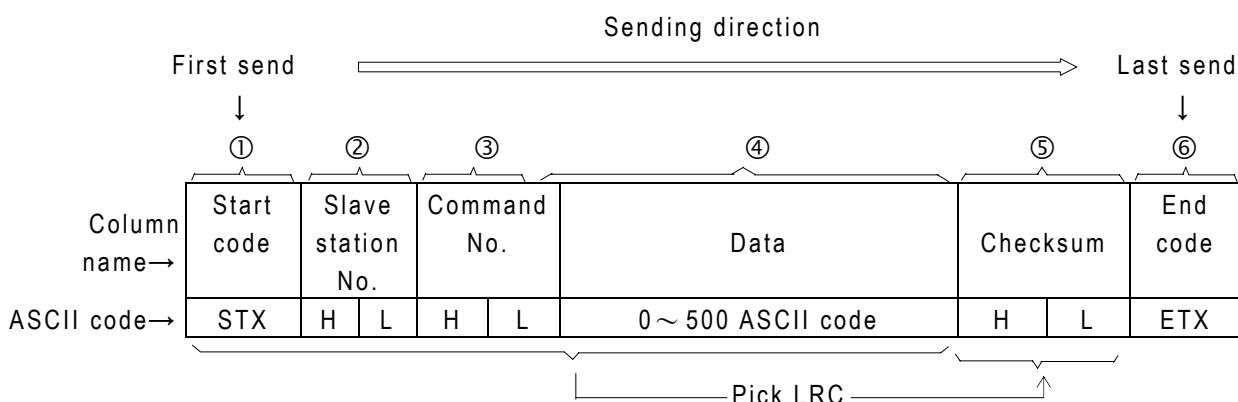
① Start code (STX) : The hexadecimal code of the STX in ASCII code is 02H. The start characters are all STX in command and response message. The receiving site can determine the data start code with STX.
