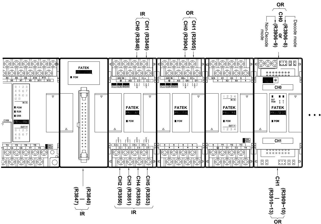
During the startup stage, FBs-PLC will automatically detect the types and CH numbers of expansion units/modules. While operation, the FBs-PLC will read the CH input values from the NI module and stores them into corresponding IR(R3804 ~ R3903) and outputs OR values (R3904~R3967) to channels on the NO module. No pre-configuration or setting by users is required.
