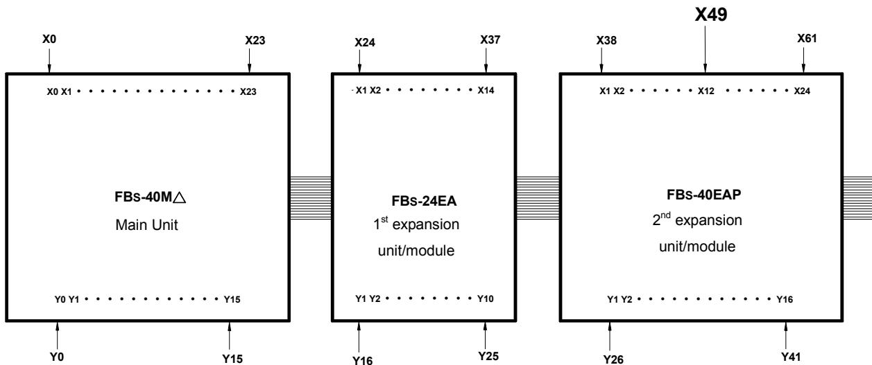
As shown in the above figure, because the top X numbers of the previous two units are 23 and 14, respectively, the number of input contact X12 on second expansion unit should be:
