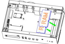
Step 2: Installing DDR3L Modules
