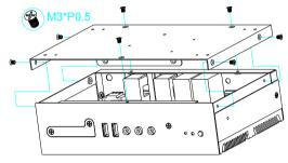
Step 1: Open the Bottom Cover (7 screws)
